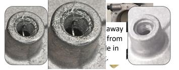
Visible wear to housing threads is expected. The new studs are significantly longer and will cut fresh threads into untouched material.
