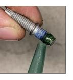
Apply one to two drops of threadlock (LOCTITE 648, supplied) to each new stud before installation (see Step 5), making sure to cover the threads completely, as shown.
