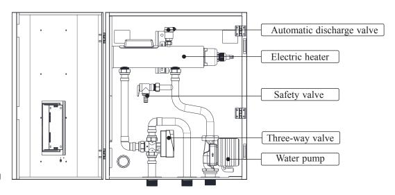
(provided by the factory). The Hydrobox requires a 208-230V power supply to operate the backup heater. Designed as a pre-piped solution, the Hydrobox simplifies installation and helps save time on the project, making it an ideal choice for installers seeking efficiency and ease of integration.
