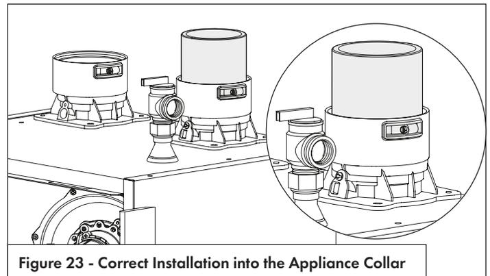
Figure 23 - Correct Installation into the Appliance Collar
