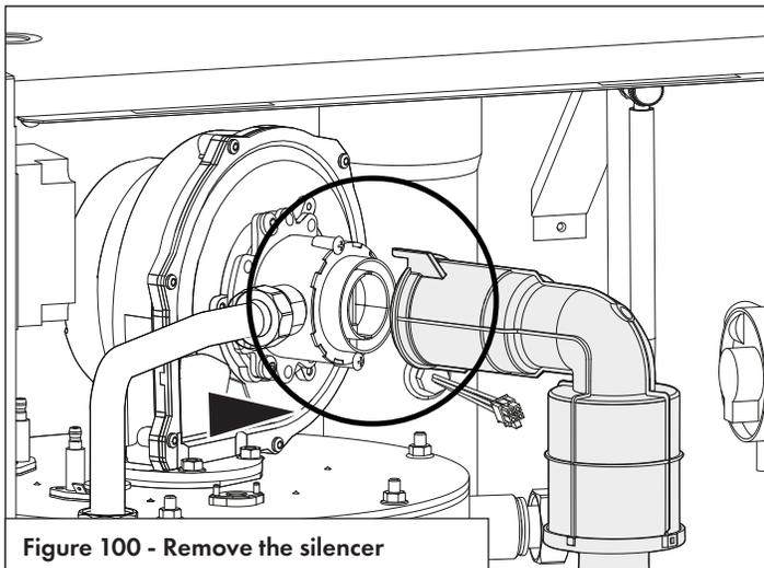
Figure 100 - Remove the silencer
