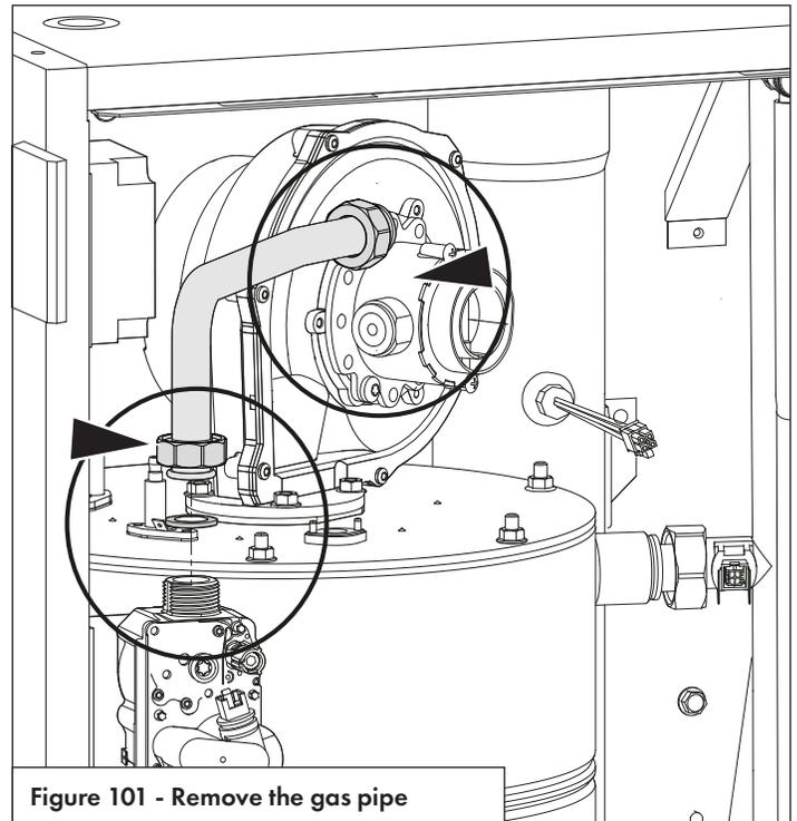
Figure 101 - Remove the gas pipe
