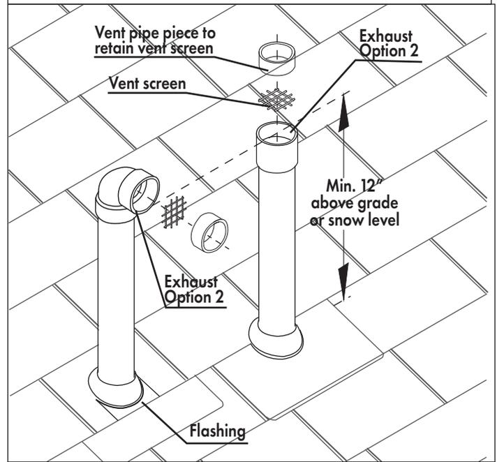
Figure 41 - Unbalanced Venting - Roof Exhaust Termination Options
