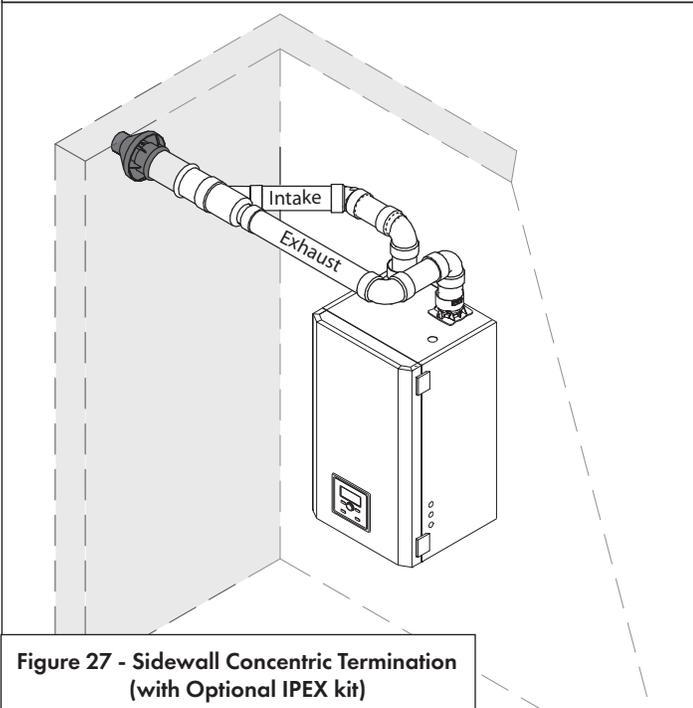
Figure 27 - Sidewall Concentric Termination (with Optional IPEX kit)
