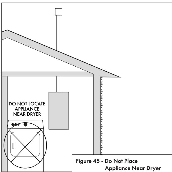
Figure 45 - Do Not Place Appliance Near Dryer
