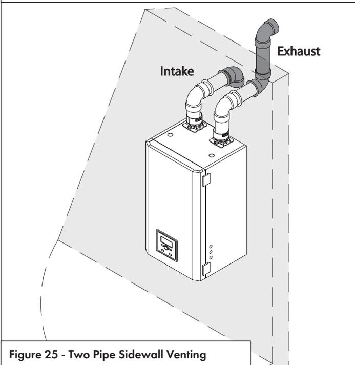
Figure 25 - Two Pipe Sidewall Venting
