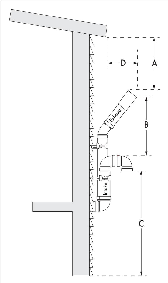
Figure 33 - Two Pipe Sidewall (Horizontal Snorkel) Venting
