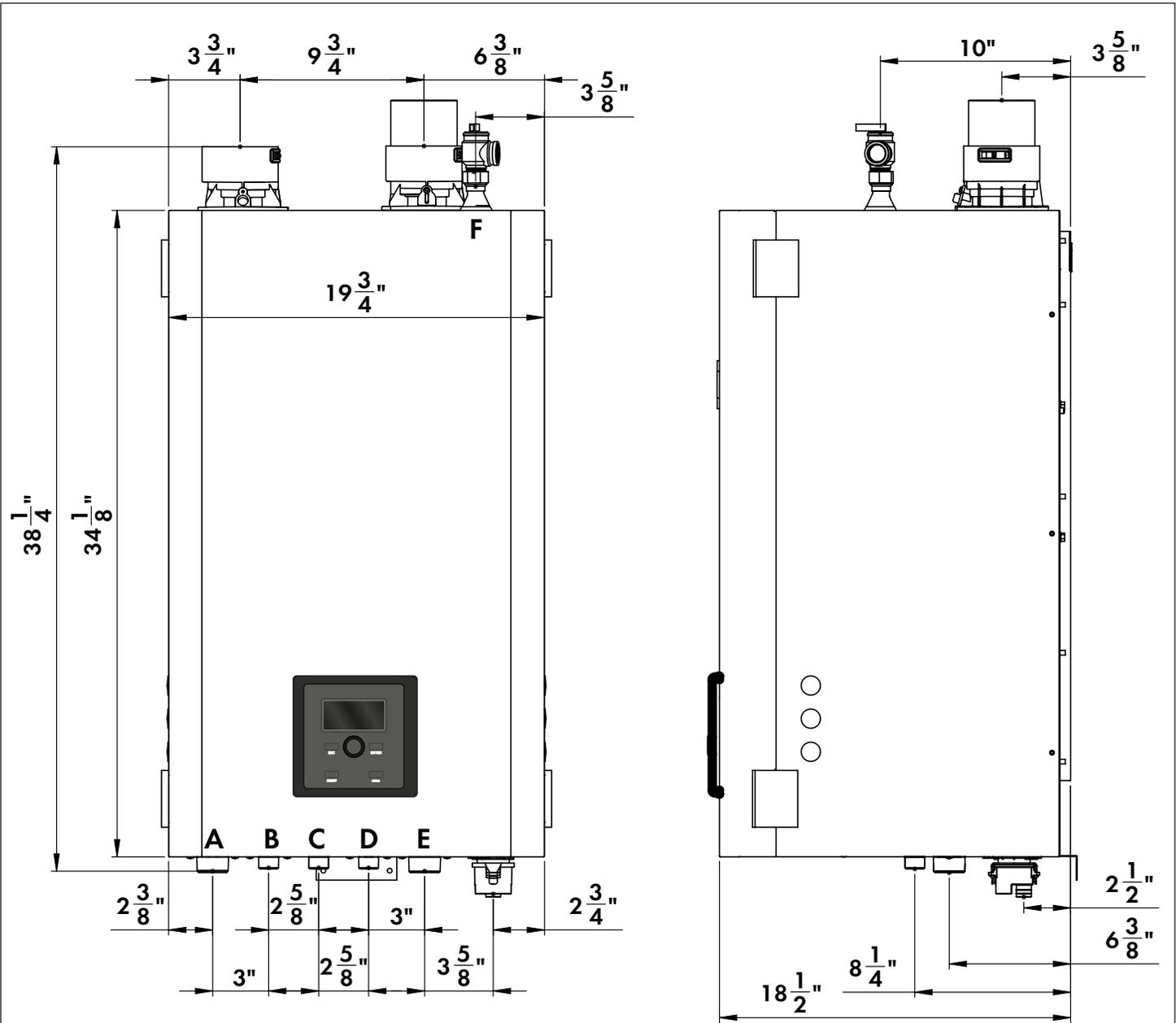
Figure 8 - Boiler Dimensions - NOTE: All Dimensions Are Approximate
