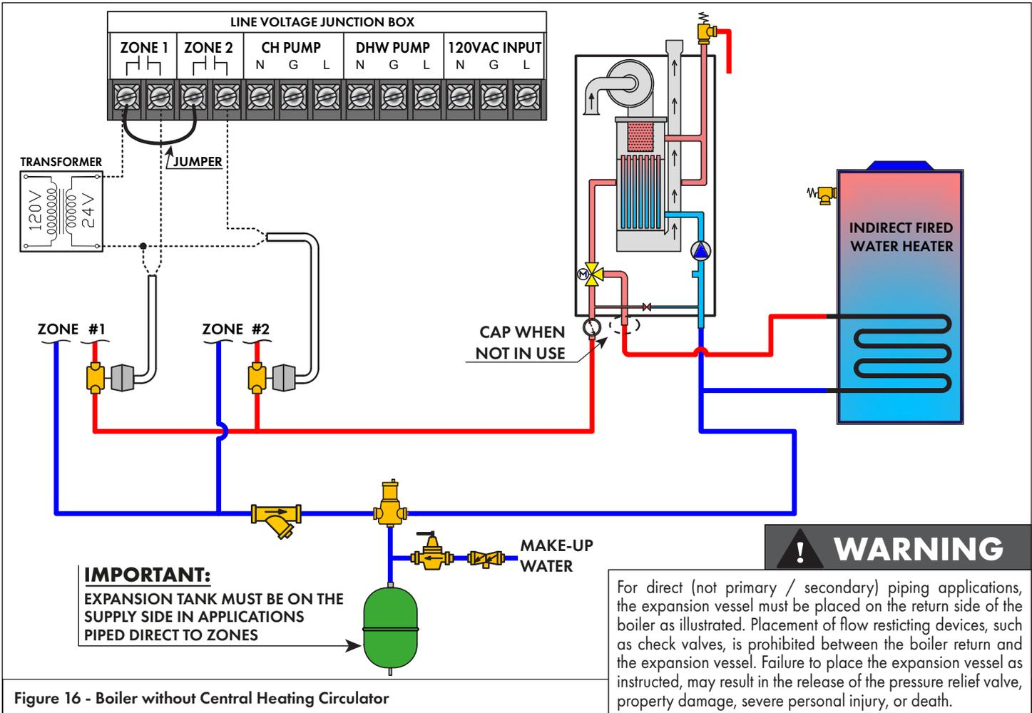
Figure 16 - Boiler without Central Heating Circulator
