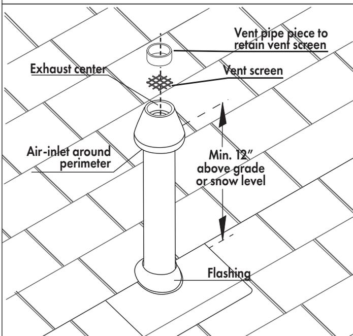
Figure 42 - Roof Concentric Termination (with Optional IPEX kit)
