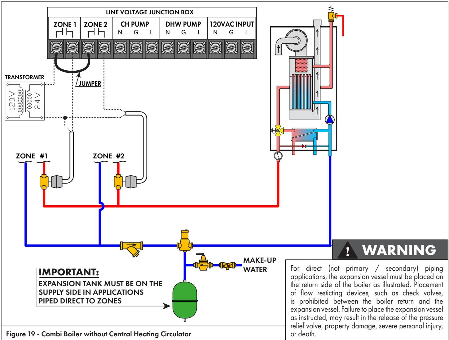
Figure 19 - Combi Boiler without Central Heating Circulator
