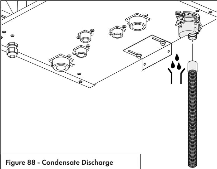
Figure 88 - Condensate Discharge
