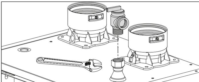
Figure 12 - Connect CH Pressure Relief Valve
