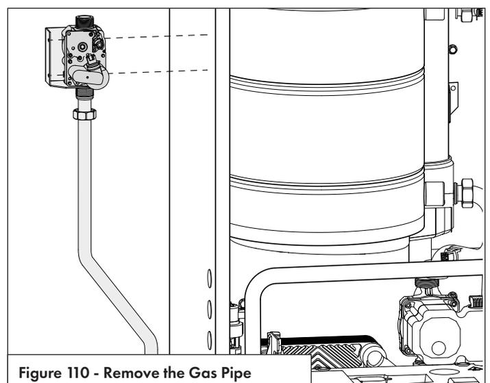
Figure 110 - Remove the Gas Pipe
