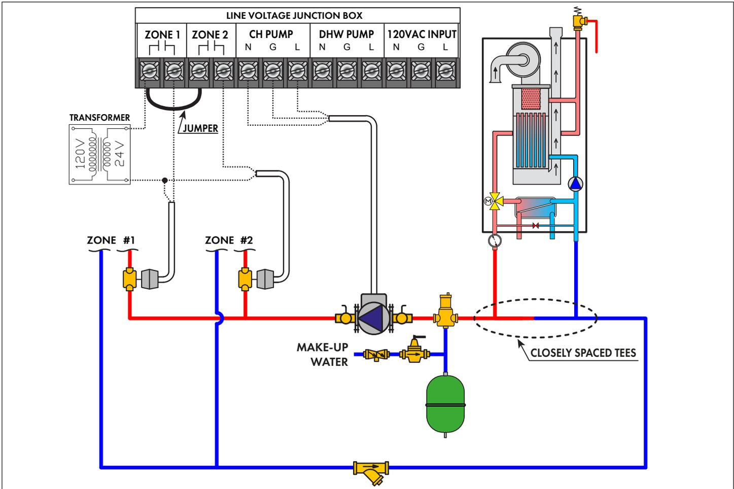
Figure 18 - Combi Boiler with Single Central Heating Circulator
