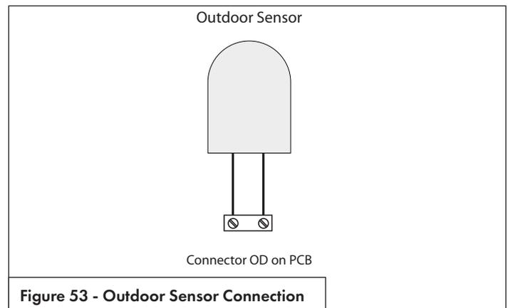
Figure 53 - Outdoor Sensor Connection
