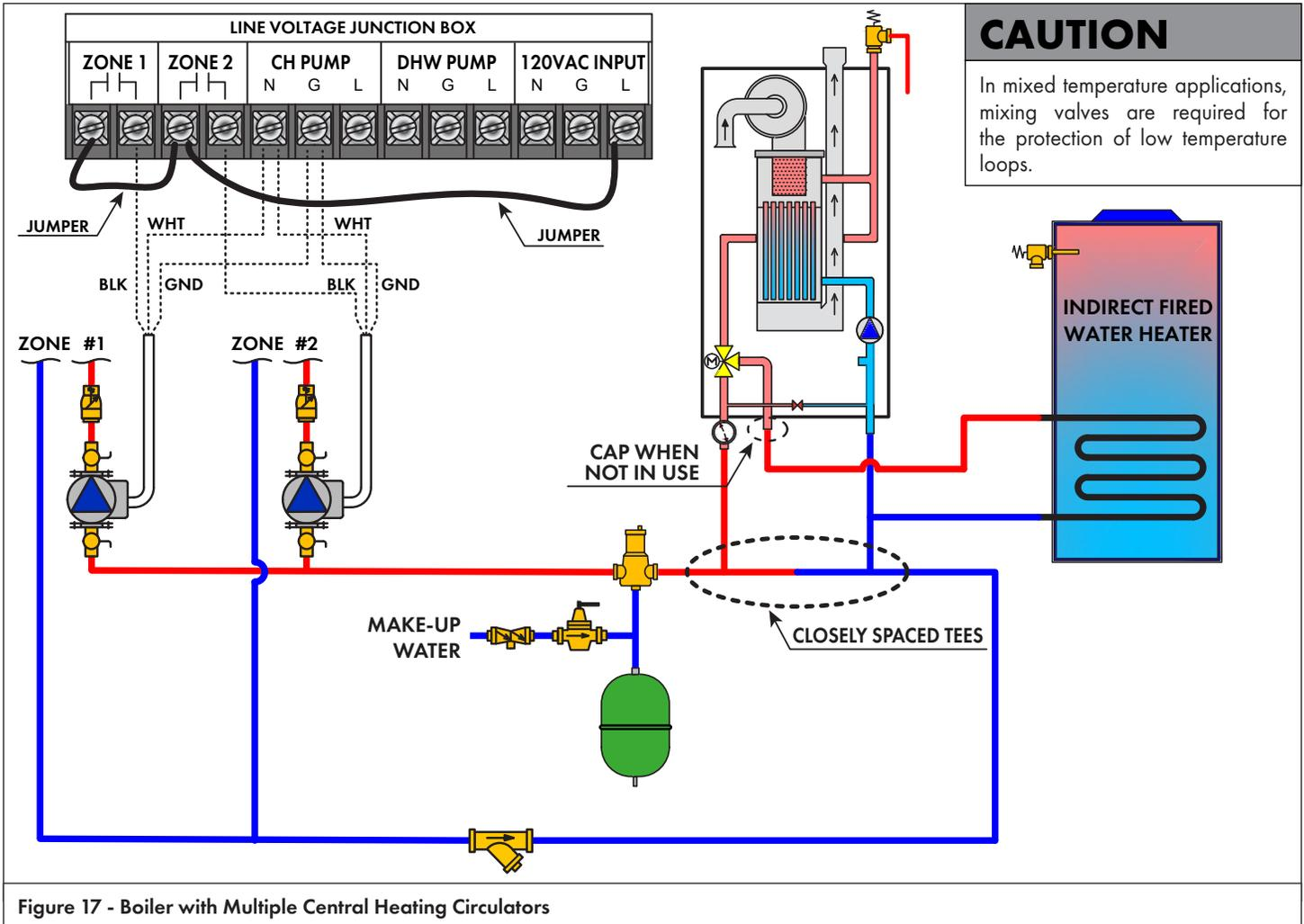
Figure 17 - Boiler with Multiple Central Heating Circulators
