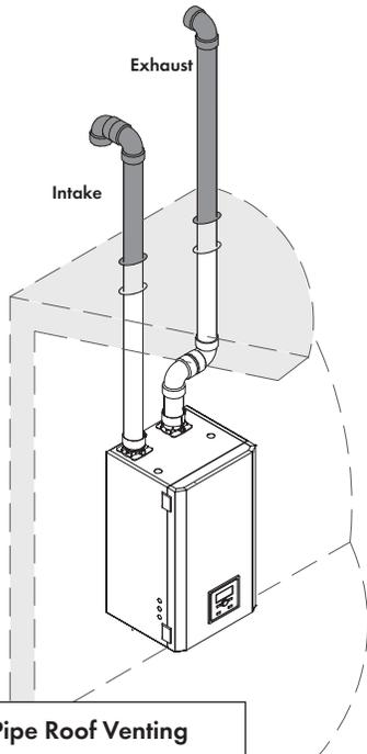
Figure 36 - Two Pipe Roof Venting
