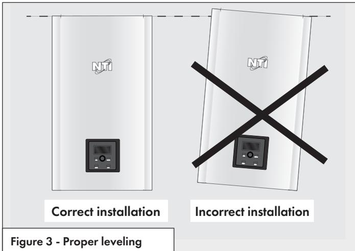
Figure 3 - Proper leveling
