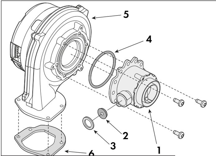
Figure 107 - Removed Fan, Mixer, and Components
