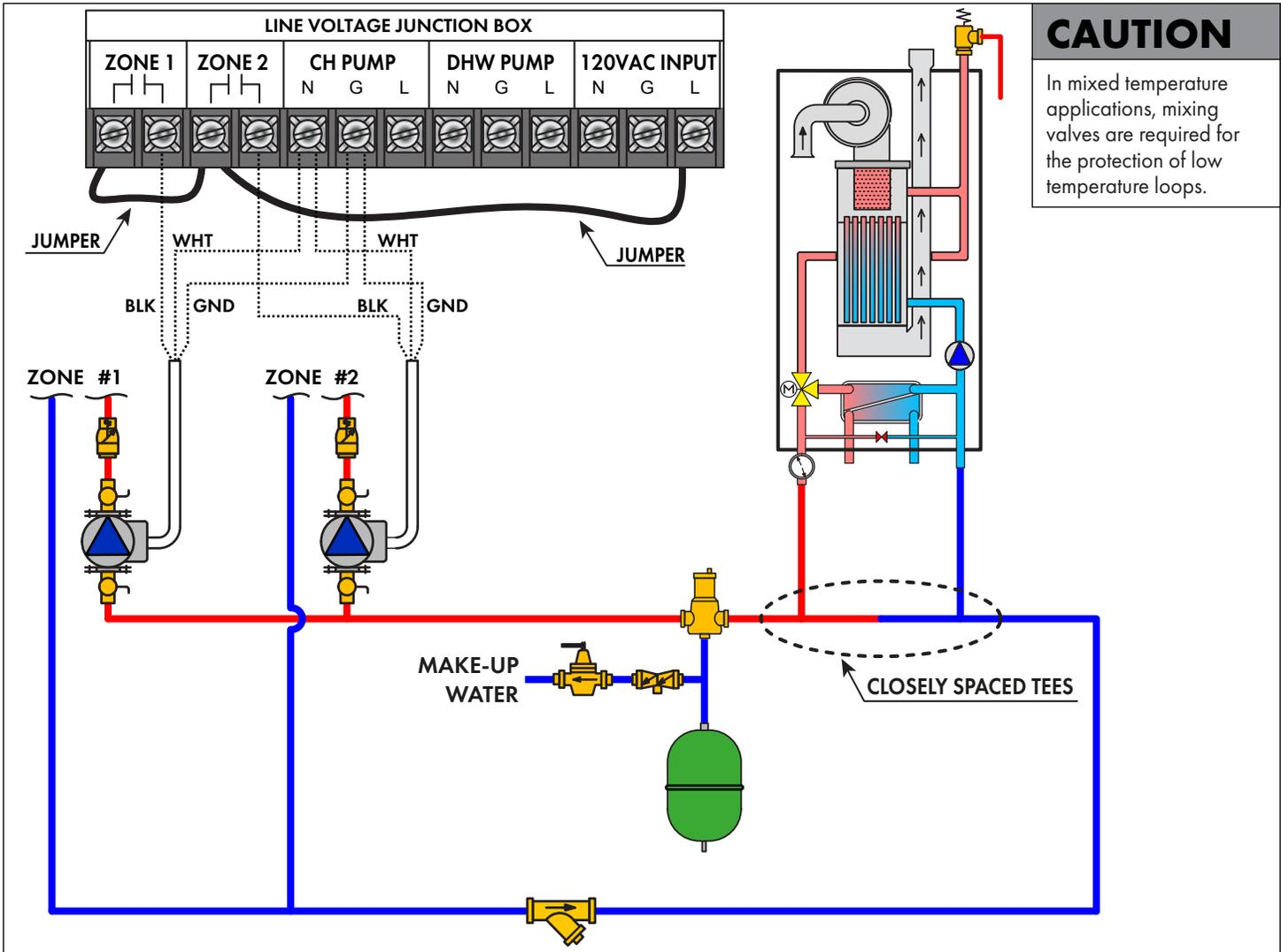
Figure 20 - Combi Boiler with Multiple Central Heating Circulators
