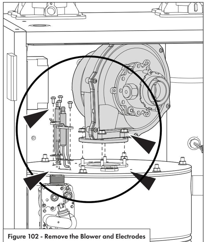
Figure 102 - Remove the Blower and Electrodes
