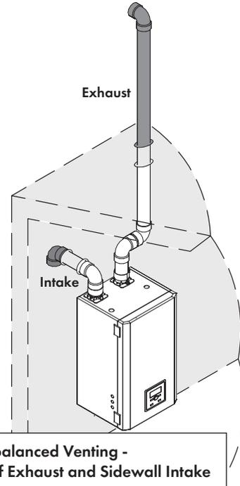
Figure 37 - Unbalanced Venting - Roof Exhaust and Sidewall Intake
