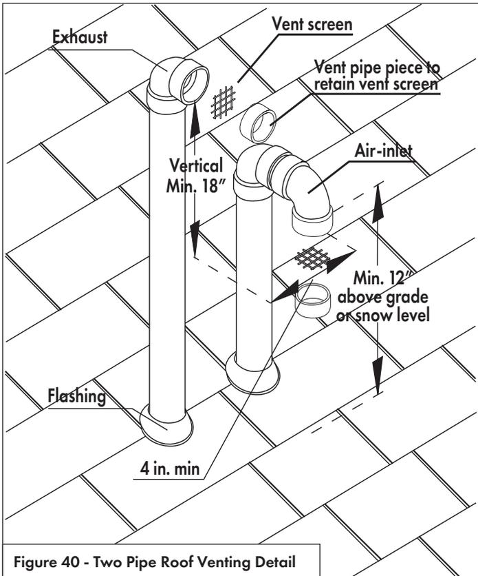
Figure 40 - Two Pipe Roof Venting Detail
