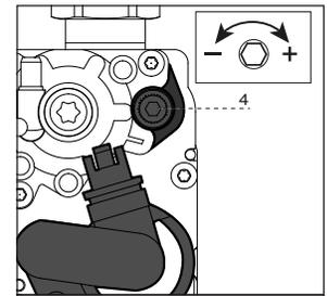
**Figure 92 - Max Power CO2 Adjustment**
