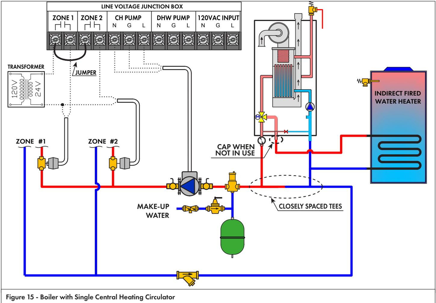
Figure 15 - Boiler with Single Central Heating Circulator
