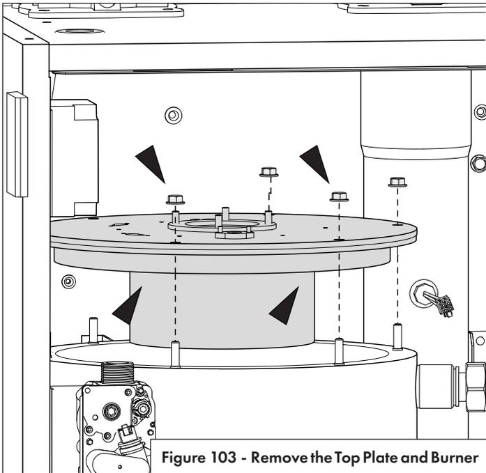
**Figure 103 - Remove the Top Plate and Burner**
