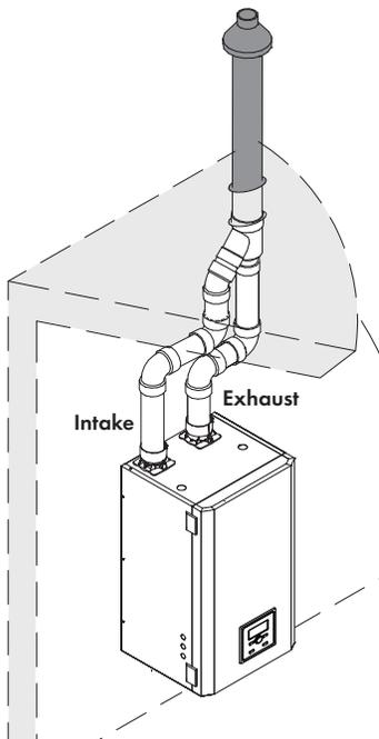
Figure 38 - Roof Concentric Termination (with Optional IPEX kit)
