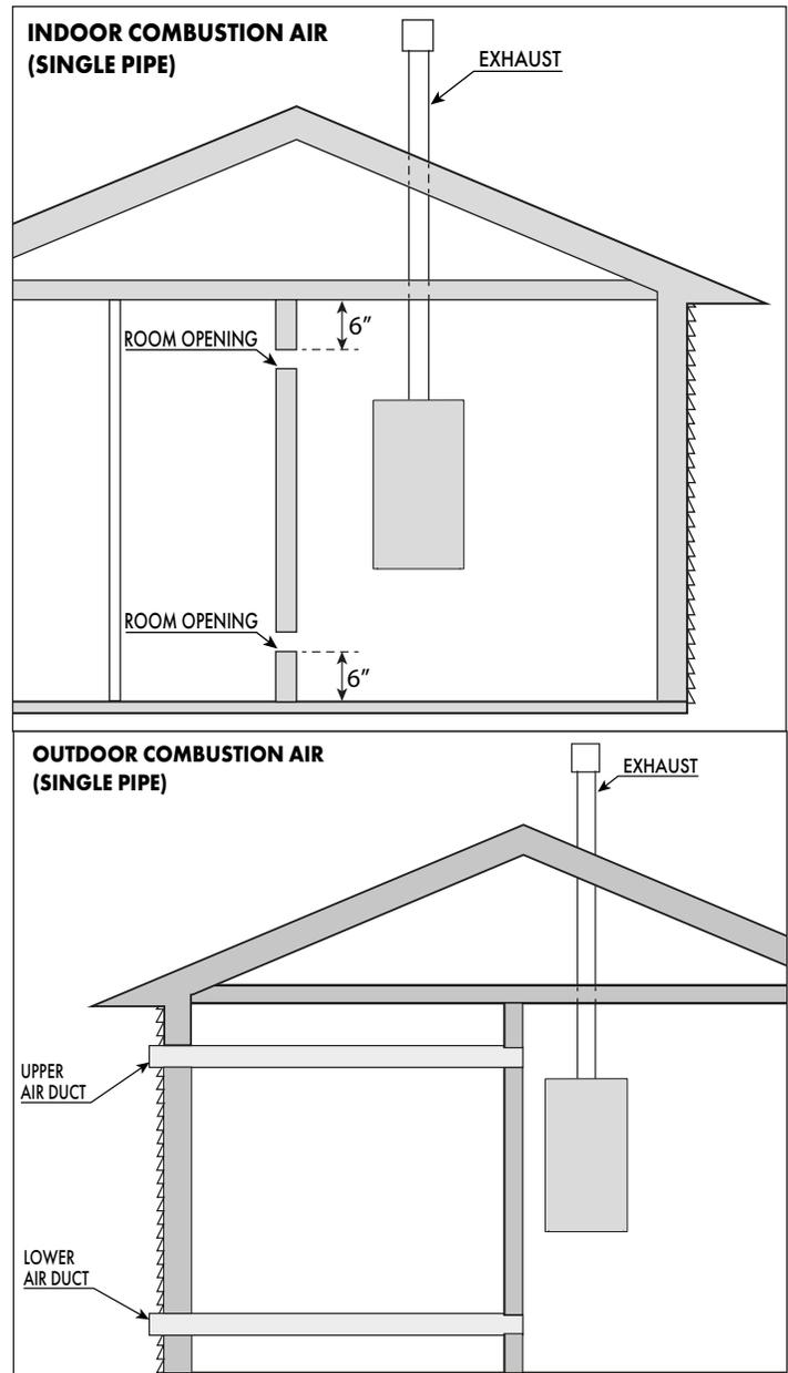
Figure 46 - Indoor and Outdoor Combustion Air - Single Pipe
