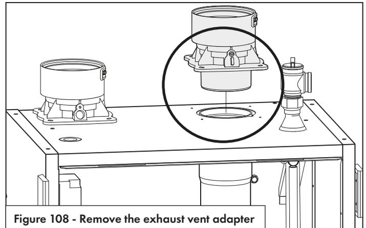
Figure 108 - Remove the exhaust vent adapter
