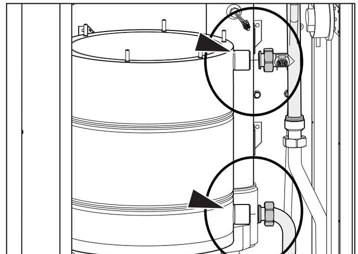
Figure 109 - Remove the CH Supply and Return Pipes
