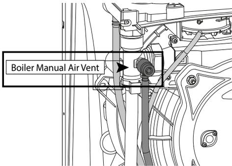
4. Open the Filling Valve (blue knob) ~ 5 turns. Water will be heard filling the boiler circuit, and air will begin to escape the vents.
