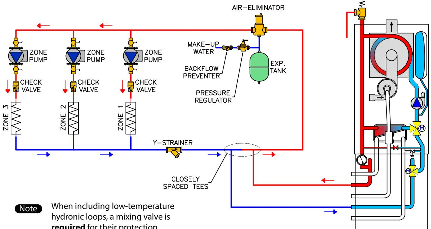
**Note** When including low-temperature hydronic loops, a mixing valve is **required** for their protection.
