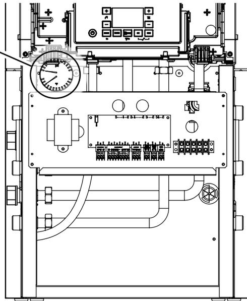
8. Continue to fill while monitoring the system pressure – NTI recommends filling the system to 20 psi.
