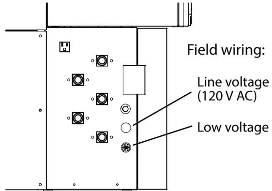
All low-voltage wiring is intended to pass through the grommet below the line voltage panel hole on either side of the cabinet.
