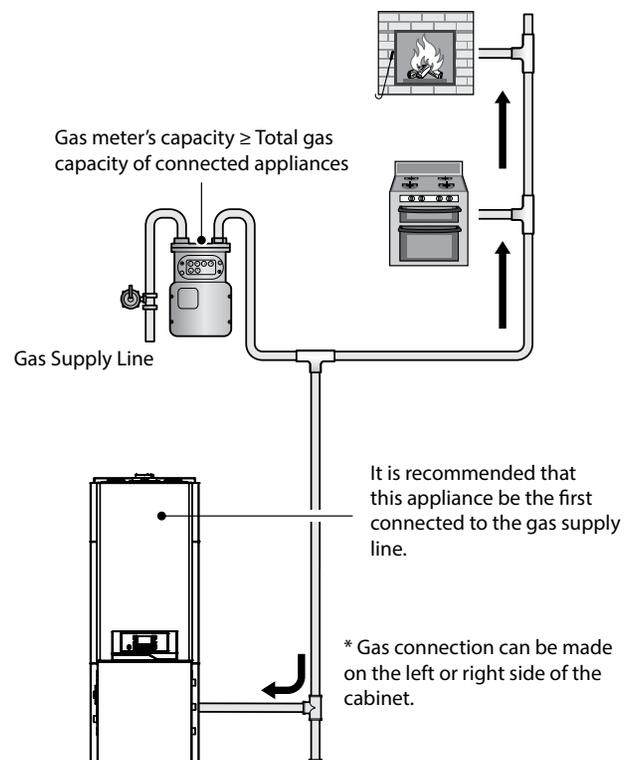
**For detailed instructions on connecting the gas supply to the appliance, see the relevant section in the boiler installation manual (supplied).**
