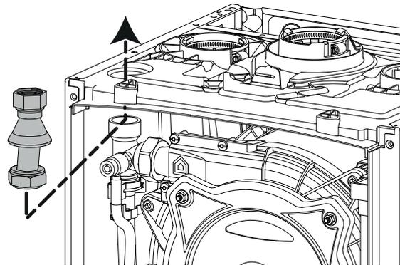
4. Connect the pressure relief valve and gasket.
