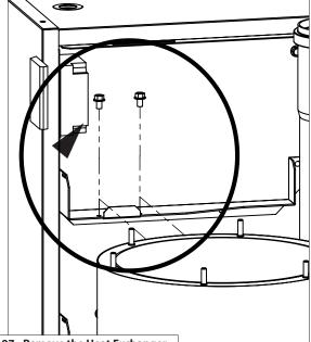
Figure 97 - Remove the Heat Exchanger
