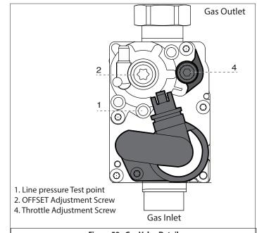
Figure 59 - Gas Valve Detail
