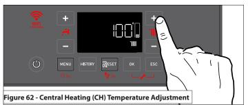
**NOTE:** When set to AUTO - Automatic Temperature Control (e.g., Outdoor Reset), the CH Temperature Setpoint is calculated in accordance with the type of automatic temperature control selected. The resulting setpoint can be offset/shifted up or down by pressing the CH +/- buttons from the home screen. See K. Parallel Shift of Reset Curve.
