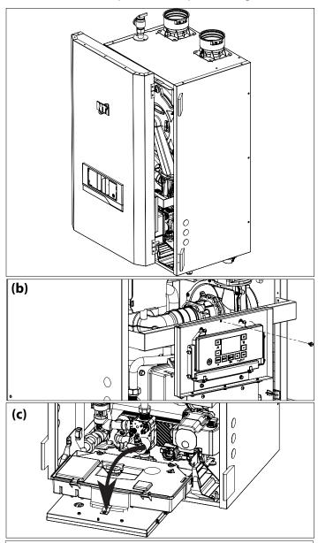
Figure 84 - Removing the Cover and Control Panel Housing
