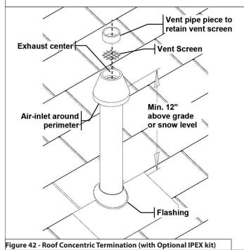
**Unbalanced Venting - Roof Exhaust Termination**
