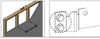
Figure 6 - Mounting the Bracket on 16" Center Studs
