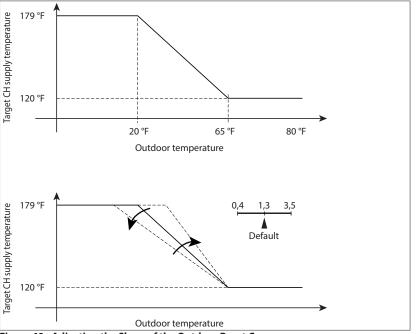
Figure 68 - Adjusting the Slope of the Outdoor Reset Curve
