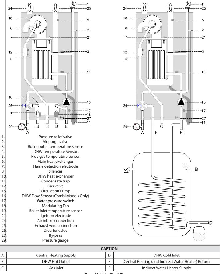
Figure 10 - Water Circuit Diagrams
