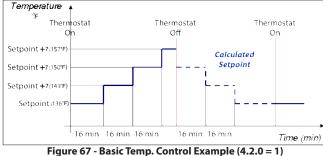
**\*\*NOTE:** The default boost interval of 16 minutes can be adjusted via parameter 2.4.4.
