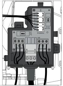
Figure 49 - 120V Connections for DHW and CH Circulators
