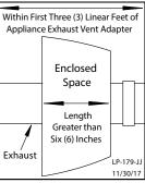
CPVC, Polypropylene, or Stainless Steel pipe material MUST be used if the first three (3) linear feet of the exhaust vent run passes through
