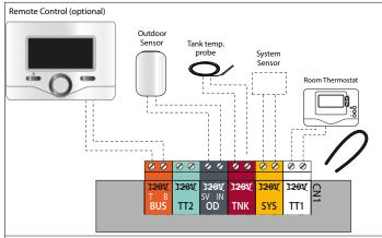
Figure 52 - Low Voltage Wiring Connections
