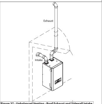
Figure 37 - Unbalanced Venting - Roof Exhaust and Sidewall Intake
