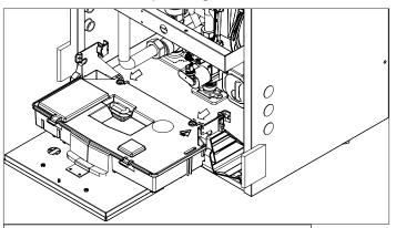
Figure 50 - Disconnecting the Two Clips
