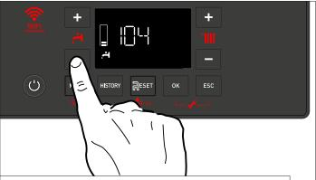
Figure 63 - Domestic Hot Water (DHW) Temperature Adjustment
