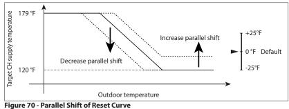
**NOTE:** Adjusting Parallel Shift is only possible when Auto Boost is OFF (4.7.5 = 0).
