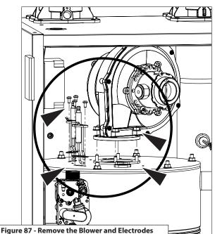
6. Remove the six (6) lock nuts securing the top plate to the heat exchanger. Remove the top plate and burner.
