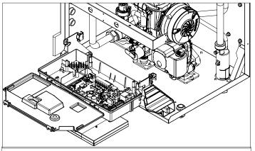
Figure 49 - Access to Low Voltage Wiring Connections
