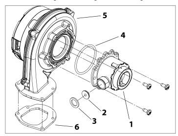
Figure 89 - Removed Fan, Mixer, and Components
