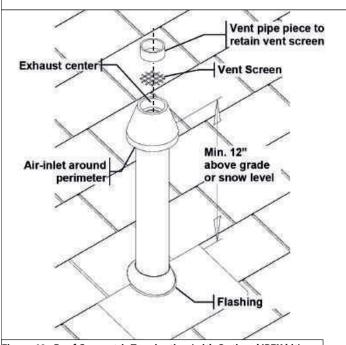
Figure 40 - Roof Concentric Termination (with Optional IPEX kit)
