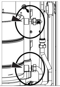
Figure 91 - Remove the CH Supply and Return Pipes
