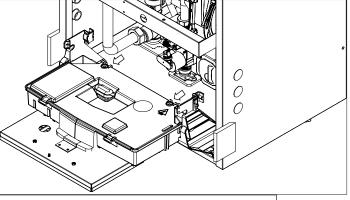
Figure 48 - Disconnecting the Two Clips
