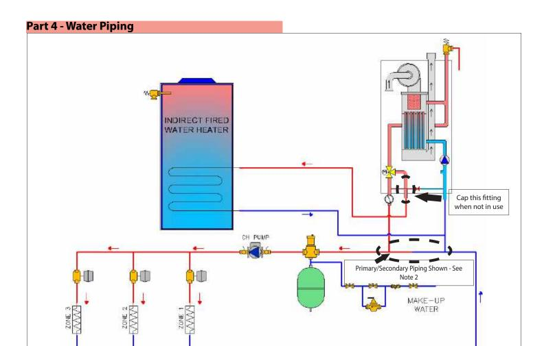
**NOTE:** In piping applications utilizing a single zone, it is recommended that the installer use flow / check valves with weighted seats at or near the appliance to prevent gravity circulation.
