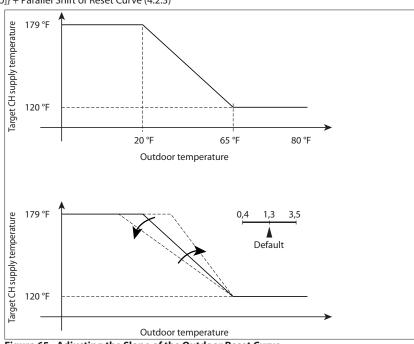
Figure 65 - Adjusting the Slope of the Outdoor Reset Curve
