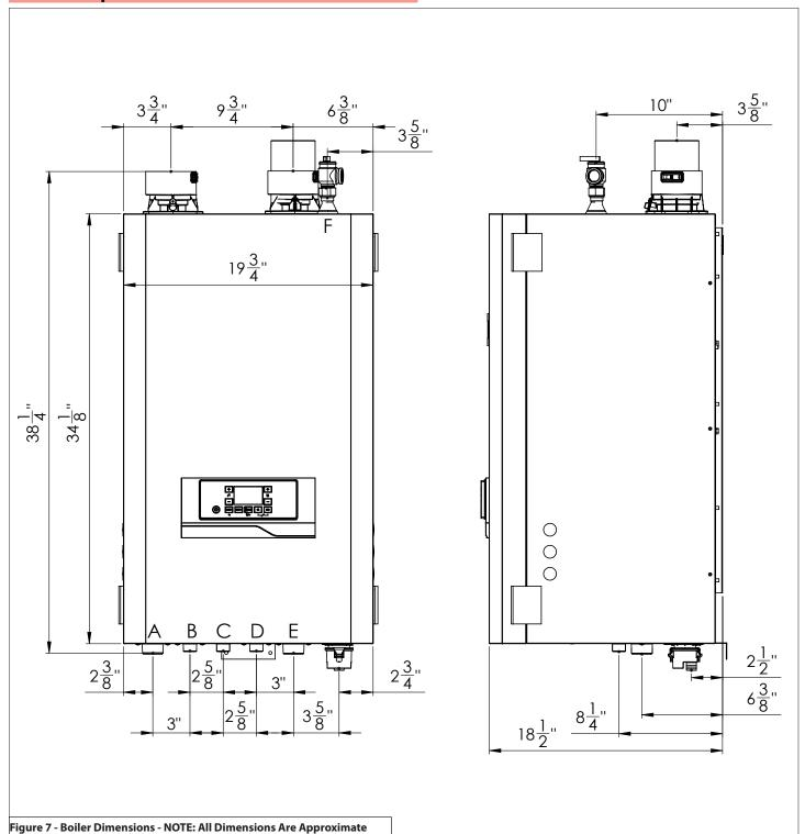
Model **Non-Combi Models** Model **Combi Models A - Central Heating Supply** A - Central Heating Supply 1 1/4" NPT 1 1/4" NPT **B** - Supply to Indirect Water Heater 3/4" NPT **B - Domestic Hot Water Outlet** 3/4" NPT 3/4" NPT C - Gas Inlet C - Gas Inlet 3/4" NPT N/A **D - Domestic Hot Water Inlet** 3/4" NPT **E - Central Heating Return** 1 1/4" NPT **E - Central Heating Return** 1 1/4" NPT F - Pressure Relief Valve 3/4" NPT F - Pressure Relief Valve 3/4" NPT
