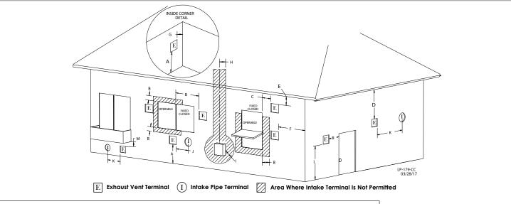
Figure 20 - Exit Terminals for Direct Vent Systems - ANSI Z223.1 / NFPA 54 for US and CAN/CSA B149.1 for Canada
