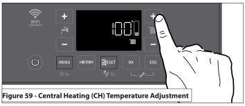
NOTE: When set to AUTO - Automatic Temperature Control (e.g., Outdoor Reset), the CH Temperature Setpoint is calculated in accordance with the type of automatic temperature control selected. The resulting setpoint can be offset/shifted up or down by pressing the CH +/- buttons from the home screen. See K. Parallel Shift of Reset
