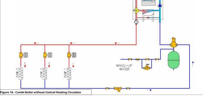
**NOTE:** In piping applications utilizing a single zone, it is recommended that the installer use flow / check valves with weighted seats at or near the appliance to prevent gravity circulation.
