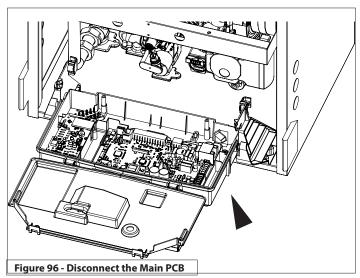
Follow the instructions provided with the replacement PCB kit for setting all necessary parameters.
