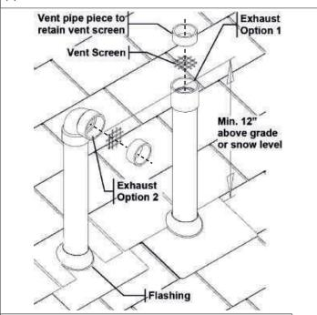
Figure 39 - Unbalanced Venting - Roof Exhaust Termination Options
