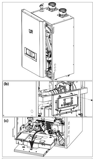
Figure 81 - Removing the Cover and Control Panel Housing
