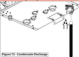
If the condensate outlet on the boiler is lower than the drain, you must use a condensate removal pump. This pump is equipped with two leads that can be connected to an alarm or another type of warning device to alert the user of a condensate overflow, which, if not corrected, could cause property damage.
