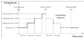
Figure 64 - Basic Temp. Control Example (4.2.0 = 1)
