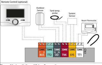
Figure 50 - Low Voltage Wiring Connections
