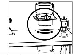
Figure 90 - Remove the exhaust vent adapter
