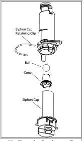
Figure 87 - Clean the Condensate Trap
