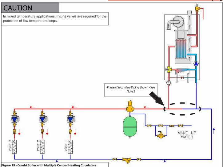
**NOTE:** In piping applications utilizing a single zone, it is recommended that the installer use flow / check valves with weighted seats at or near the appliance to prevent gravity circulation.
