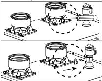
Figure 74 - Combustion Test Port
