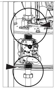
Figure 95 - Disconnect the Gas Valve
