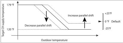
Figure 67 - Parallel Shift of Reset Curve
