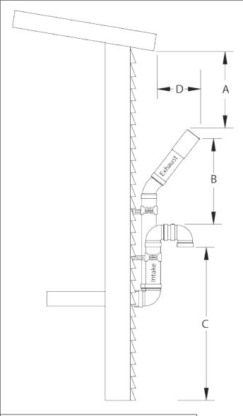
Figure 31 - Two Pipe Sidewall (Horizontal Snorkel) Venting
