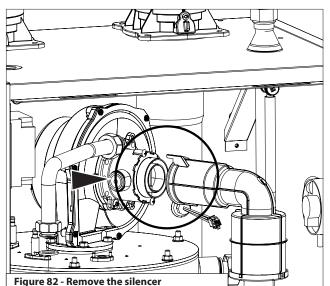
2. Unscrew the two nuts and remove the gas pipe.
