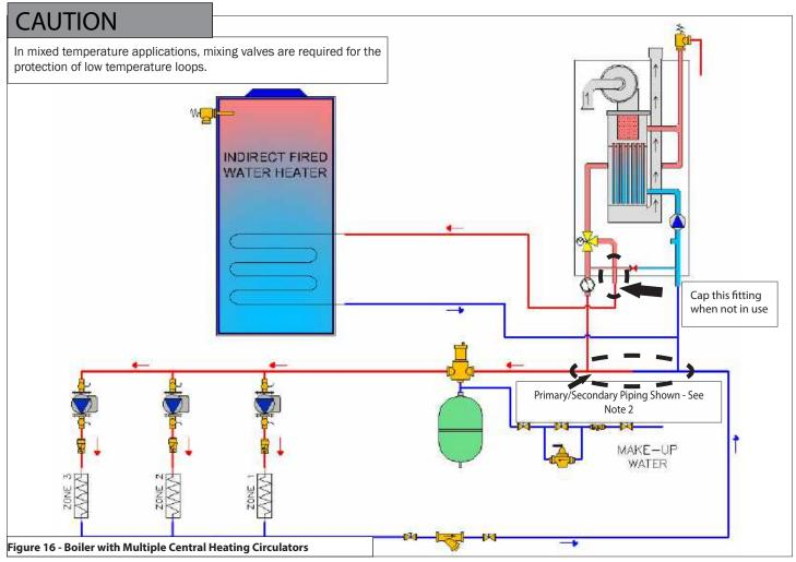
**NOTE:** In piping applications utilizing a single zone, it is recommended that the installer use flow / check valves with weighted seats at or near the appliance to prevent gravity circulation.
