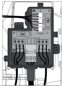
Figure 47 - 120V Connections for DHW and CH Circulators
