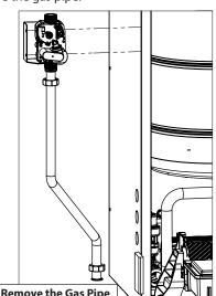
Figure 92 - Remove the Gas Pipe
