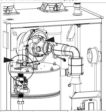
Figure 83 - Remove the gas pipe
