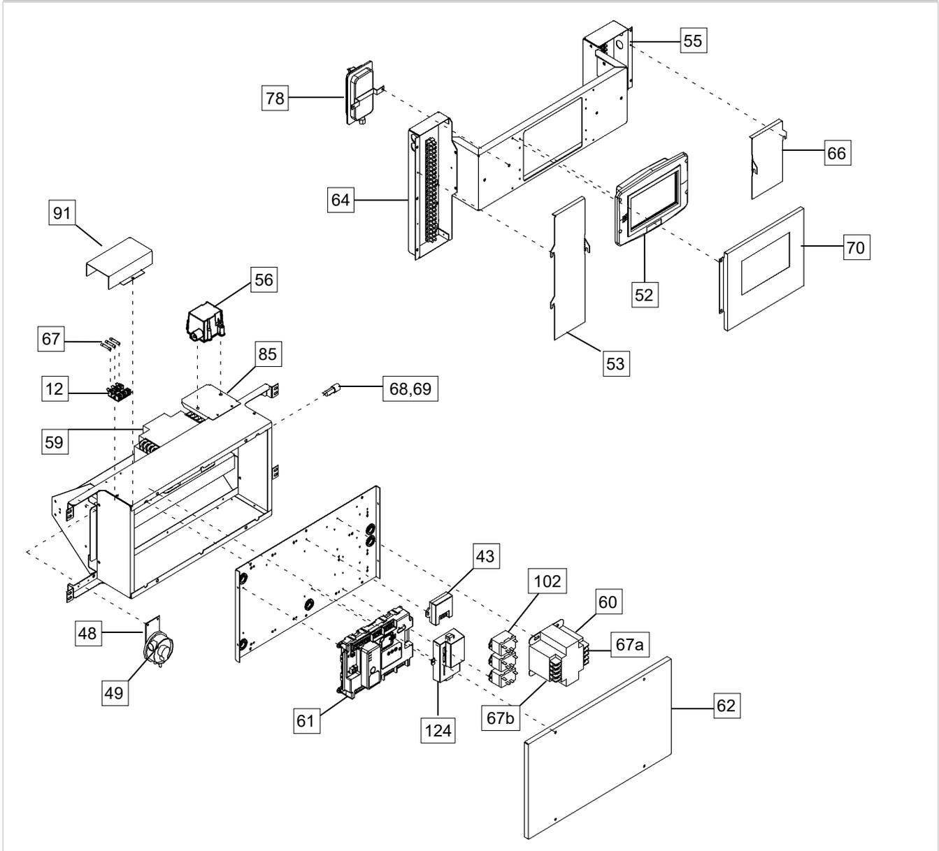
**Figure 17-1(c) Exploded View – Trim/Install Kit**
