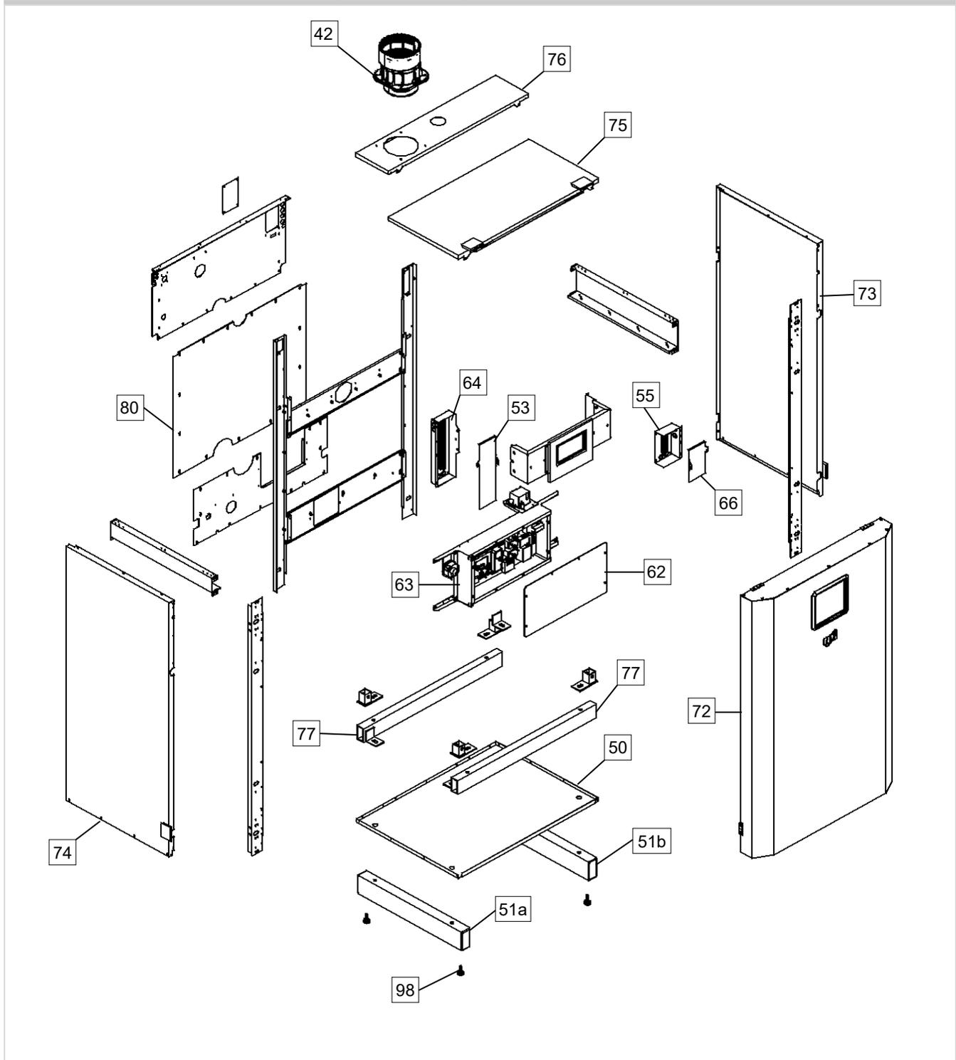
**Figure 17-1(b) Exploded View – Control Panel**
