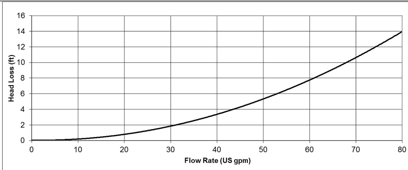
Figure 10-2(b) FTG 1200-1400 Head Loss Curve
