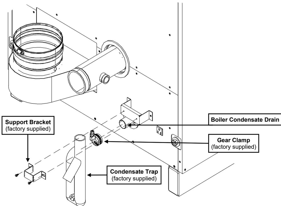
Figure 6-1(b) Condensate Drain Trap - Assembled
