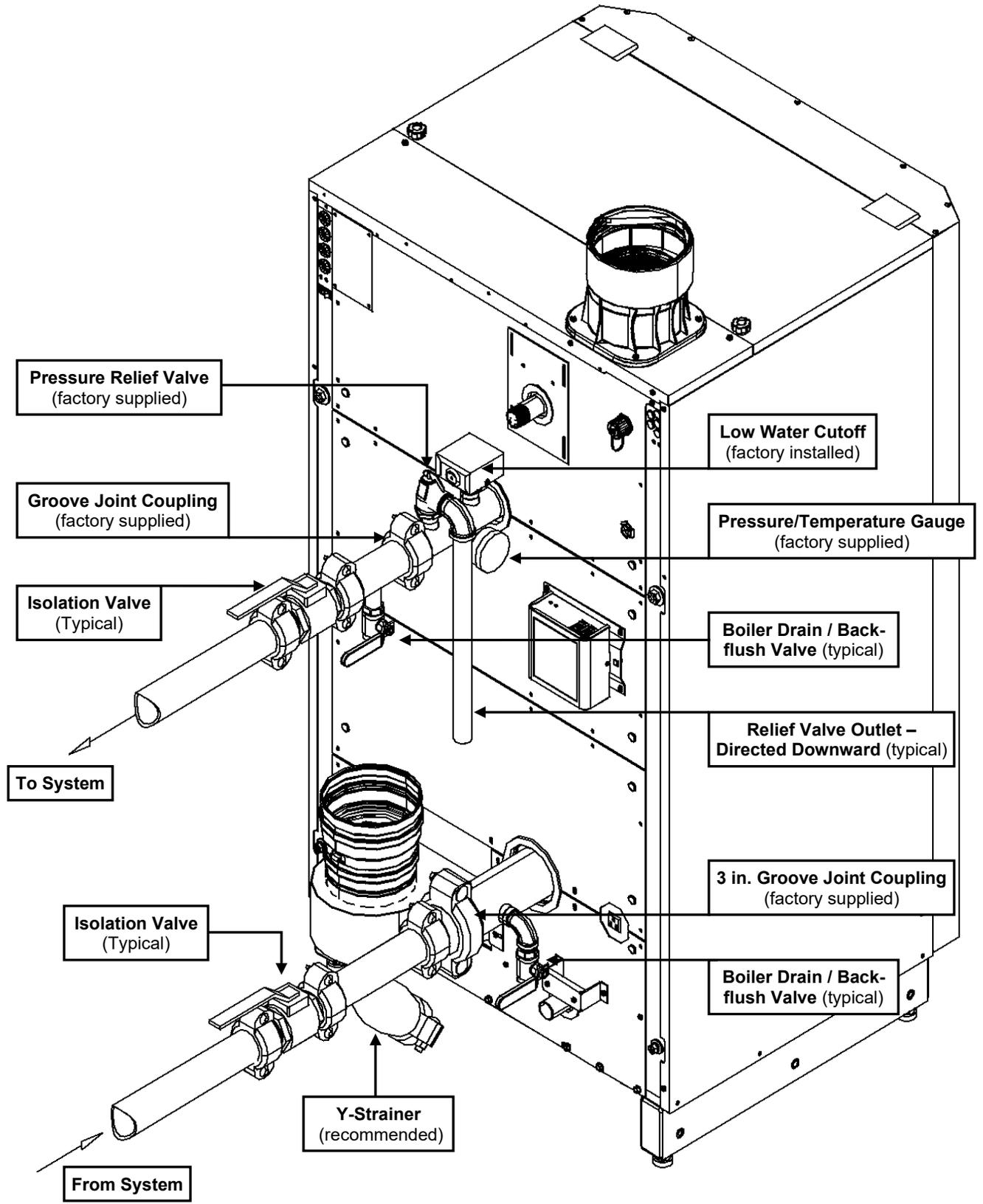
**ATTENTION:** Boiler piping can be adapted to ANSI pipe thread, flange, or other style piping connection, immediately upon exiting the boiler. With the exception of the boiler inlet and outlet fittings, Grooved Joint style piping connections are **NOT** required.
