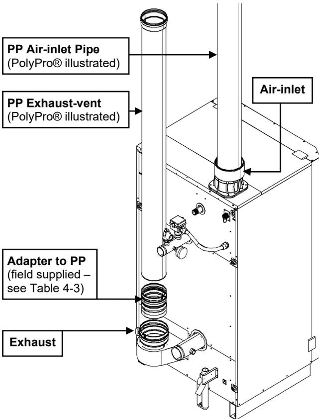
Figure 4-1(d) Near Boiler Venting (SS)
