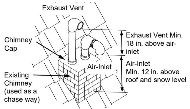
**5.0 VENT/AIR-INLET TERMINATION CLEARANCES**
