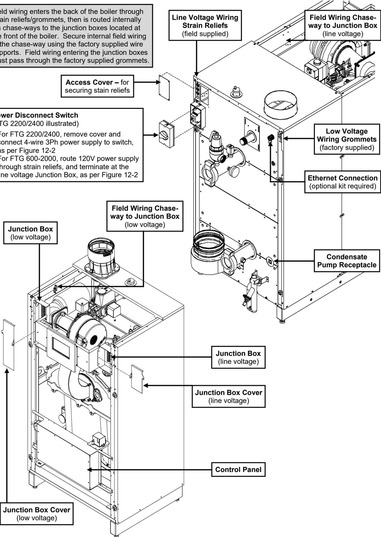
Figure 12-2 Line Voltage Field Wiring
