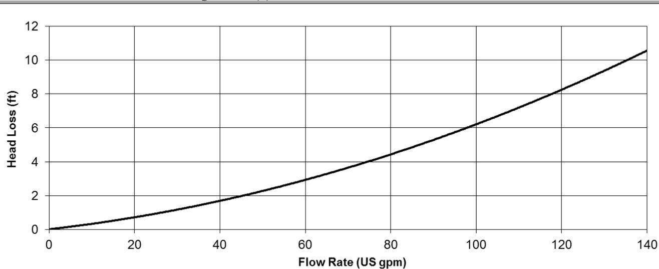
Figure 10-2(c) FTG 2000-2400 Head Loss Curve
