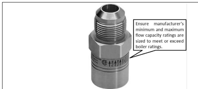
Figure 71 - Excess Flow Valve (EFV)
