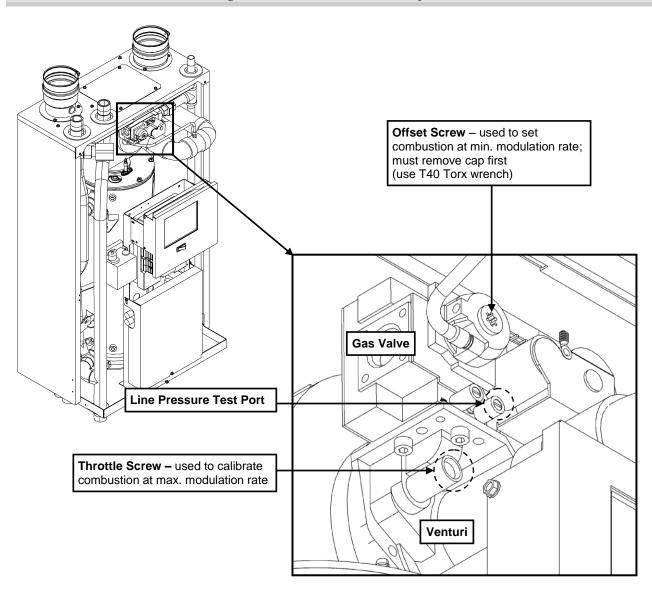
Figure 9-2 Tft154 & Tft201 Gas Valve Adjustment
