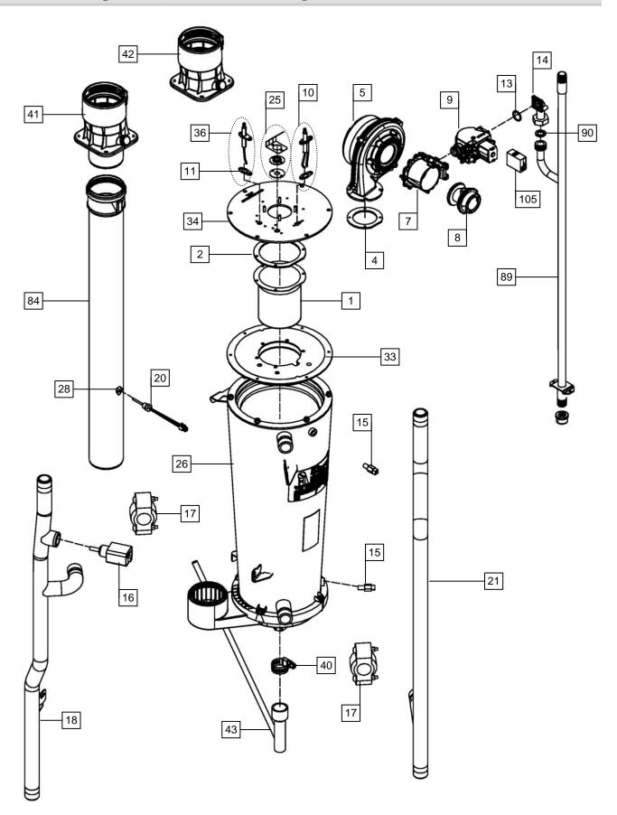
Figure 17-1(c) Tft285-399 Heat Engine and Gas Train (Tft340-399 Illustrated)
