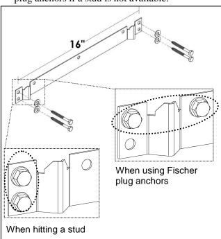
**3** With the help of an assistant, hang the boiler on the upper wall mount bracket. Align the openings in the back of the boiler with the hooks of the wall mount bracket. Make sure that it is securely hooked and that the wall mount bracket remains securely fastened to the wall.
