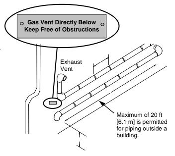
Figure 4-10 Existing Chimney Chase Way
