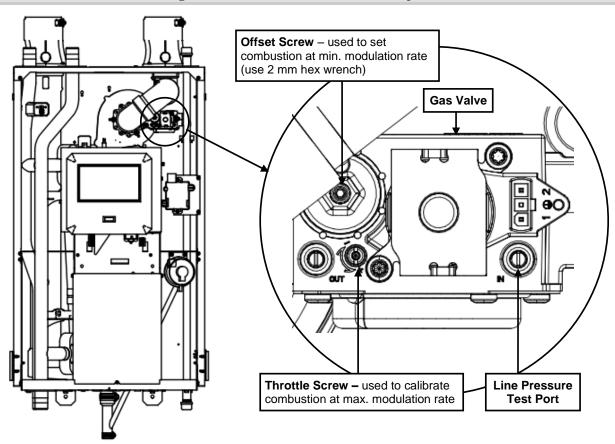
Figure 9-3 Tft285-399 Gas Valve Adjustment (Tft340-399 Illustrated)
