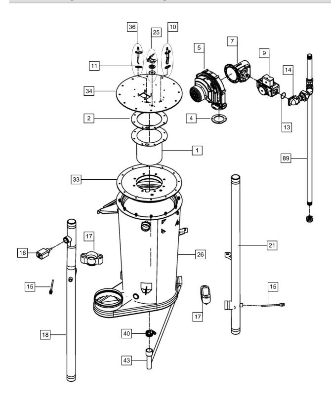
Figure 17-1(d) Tft Cabinet, Vent and Air-inlet Parts (Tft60-110 Illustrated)
