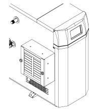
Secure the filter in place with the brackets and knurled screws provided in the filter kit.
