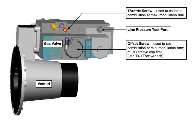
Figure 9-3 Gas Valve Assembly (Lx500)
