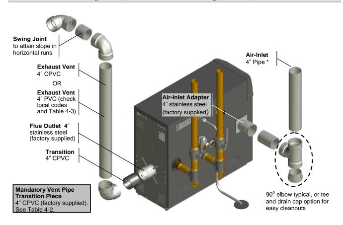
Figure 4-5(a) Lx700-800 Near Boiler Venting (CPVC)
