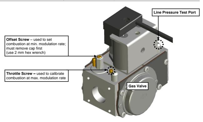
Figure 9-4 Gas Valve and Venturi Assembly (Lx600-Lx800)
