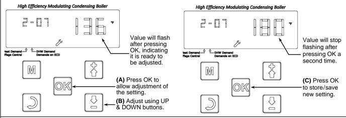
**STEP 6 – DHW MODE:** Press the UP button to advance to Installer setting 2-08, DHW mode; default setting = 2 (5 for Combi). Adjust setting as described in STEP 3. *Note: set value according to the application needs, e.g. choose 1 when using a tank sensor; choose 2 when using a tank thermostat; (must choose 5 for Combi models; 1 for Vmax Plus models)*
