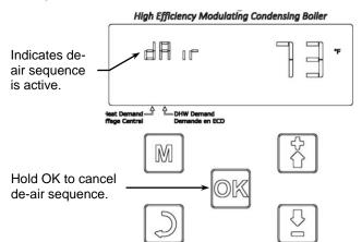
STEP 2 – ACCESS INSTALLER MENU: Access the Installer Menu by pressing and holding the MENU and OK buttons at the same time until 2-01 is displayed in the top left corner of the display – see STEP 3.
