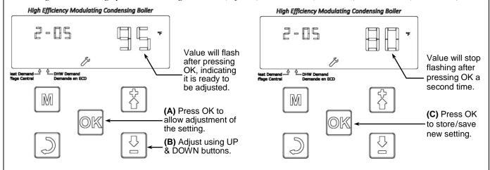
**STEP 5 – DHW SETPOINT:** By pressing the UP button, advance to Installer setting 2-07, DHW setpoint; default setting = 136°F. Adjust setting as described in STEP 3 above. *Note: set value according to the application needs, e.g. 120-140°F (Combi boiler or tank sensor); 170-190°F (tank thermostat).*
