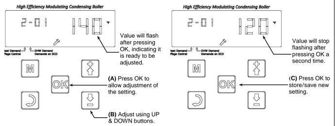
**STEP 4 – WARM WEATHER CH SETPOINT (at 70°F):** Press the UP button to advance to Installer setting 2-05, warm weather CH setpoint; default setting = 95°F. Adjust setting as described in STEP 3. *Note: set value according to the heating system needs, e.g.* 70-90°F (infloor); 100-120°F (cast-iron); 110-140°F (baseboard).
