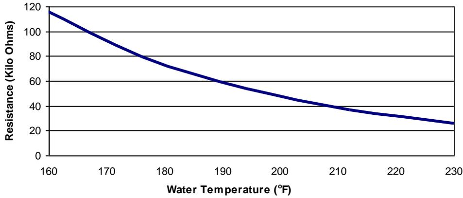
Figure 18-3 Thermistor Resistance Chart – 10 kOhm Outdoor Sensor
